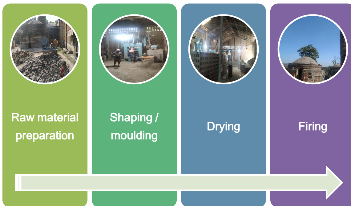
Figure 4.1: Typical production process in a refractory industry
